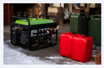
Take care when using a generator. Always isolate your generator from REC's power lines. Connect appliances or other devices directly to the generator with the appropriate cords. If you connect it directly to your building's wiring, a transfer, double-throw switch is required to separate your generator from the Co-op's system. Need assistance with properly installing a generator? REC can help.
